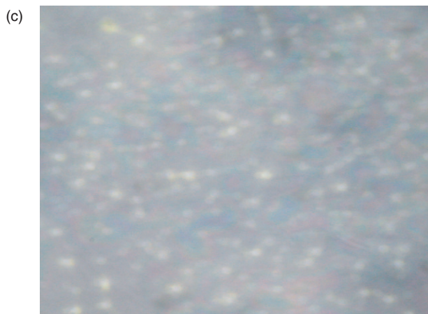
Figure 2. The CVs (a) and the relationship of anodic peak current with assembling time (b) of silver nanoparticles in the liquid membrane trapping process and (c) is the metallic microscopic image of the silver nanoparticles trapped in methyl silicone oil membrane supported on glass plate (Olympus, made in Japan, magnification \times 1200 ). Scan rate: 50 mV/s; t (min): 1, 0; 2, 12.3; 3, 17.9; 4, 30.2; 5, 39.8; 6, 50.0; 7, 54.3.
